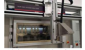
High throughput, high quality fatigue crack growth characterization
