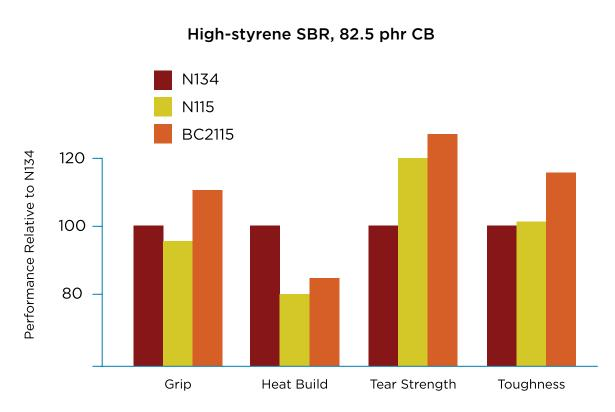
BC2115 exhibits higher levels of grip and durability while keeping heat buildup low.
